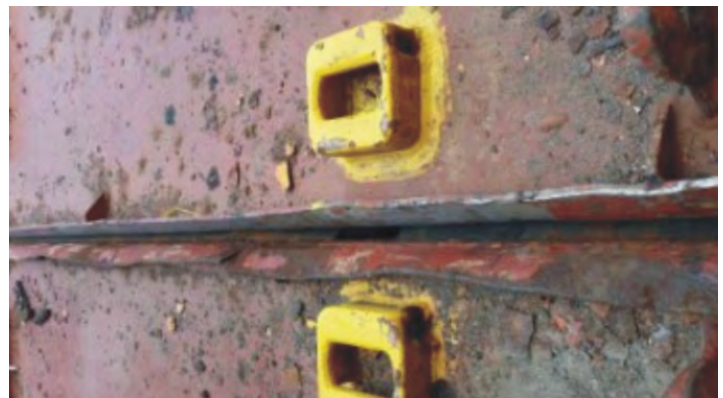
Cargo Hatch Cover Joint Gasket Damage
