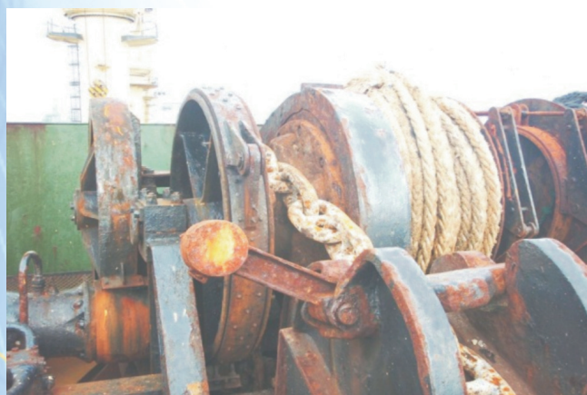
WINDLASS AND GYPSY HEAVILY CORRODED
