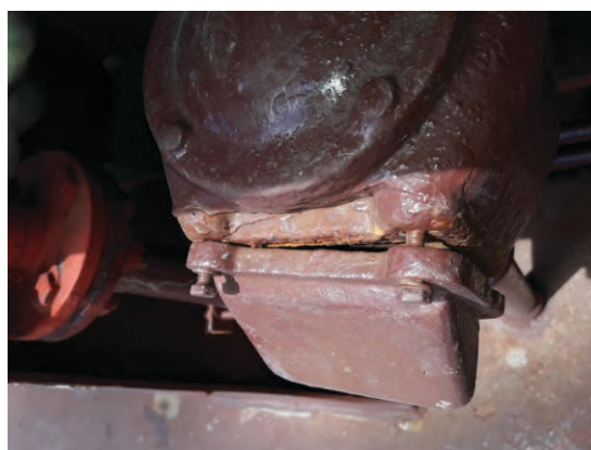
Damaged ventilator pipe on weather deck
