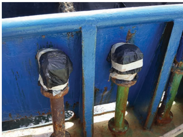
corroded air pipe vent heads (covered with plastic bags)
