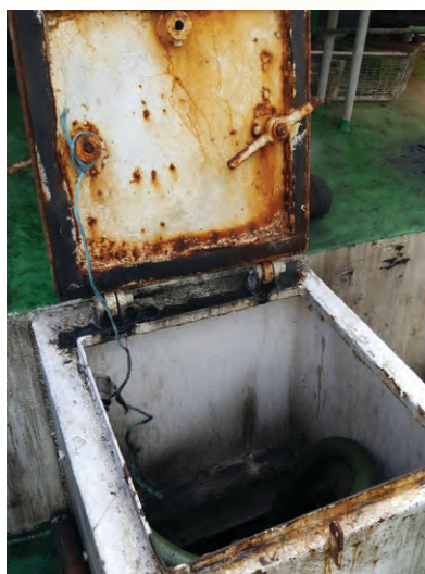
deck weathertight hatch cover with two missing dogstoggles
