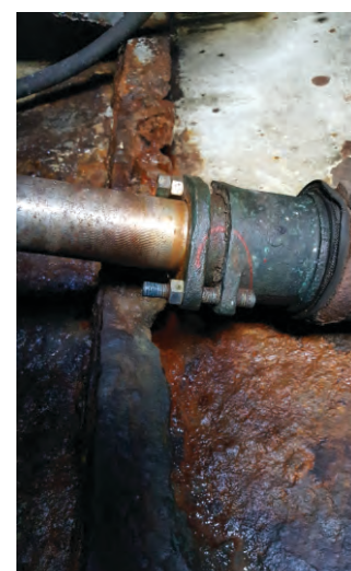
leaking stern gland and wasted shell angle framing below
